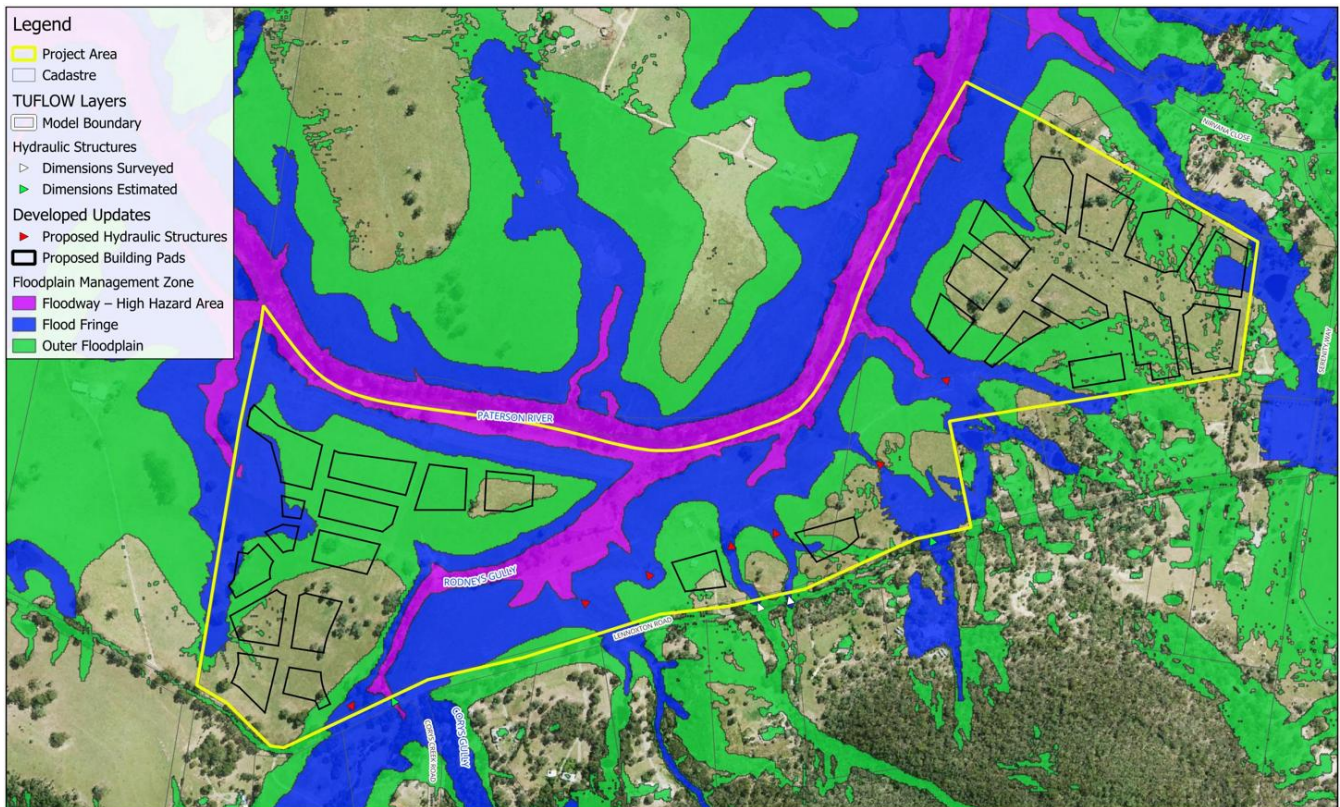
Figure 2: Floodplain management zones (Source: Engeny 2025)
